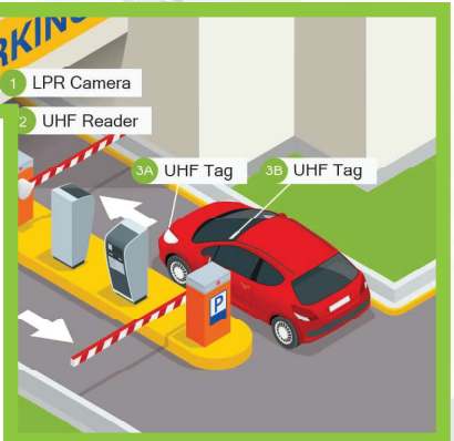
Automatic Ticket Dispensing Car Parking Management System
